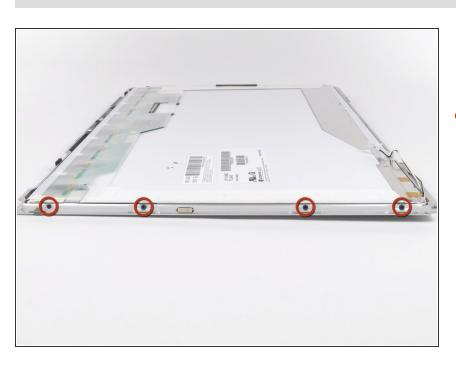
Remove the four 3.2 mm Phillips screws along the right edge of the display.
