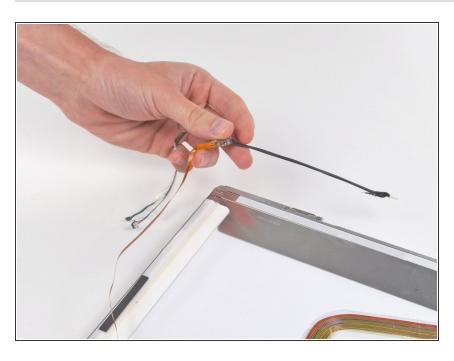
Remove the inverter/antenna cables from the display.
