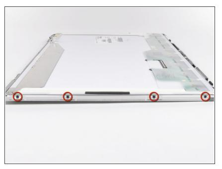
Remove the four 3.2 mm Phillips screws along the left edge of the display.
