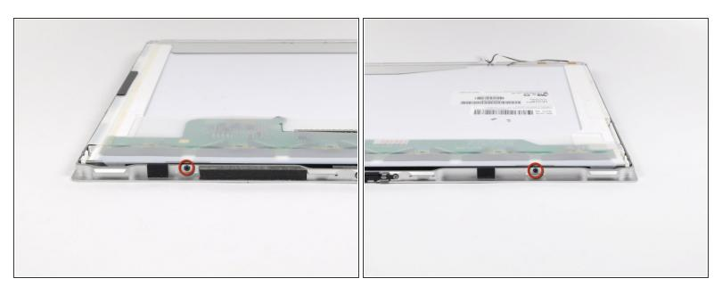
Remove the two 3.2 mm Phillips screws on the top edge of the display.
