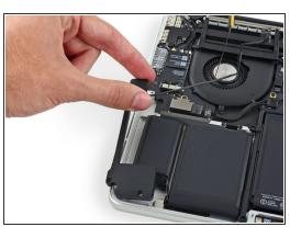
• Lift the right speaker from the cable end and pull it free from the case.
