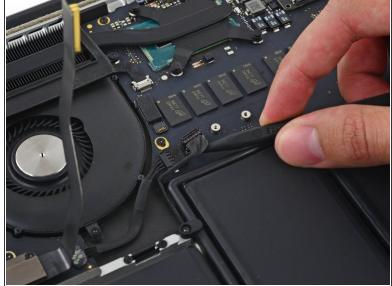
Carefully tuck the tip of a spudger under the right speaker cable near the connector and lift it up out of its socket on the logic board.
