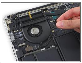
Carefully peel the right speaker cable off the upper case.
