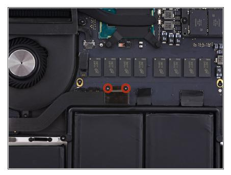
Remove the two 2.1 mm T5 Torx screws securing the logic board end of the I/O board cable bracket.
