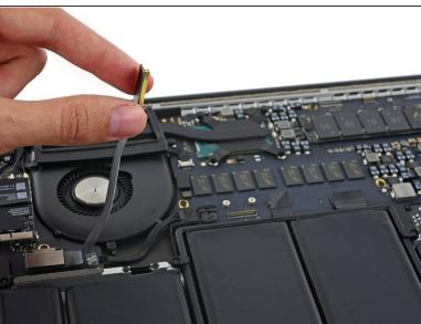
Lift the logic board end of the I/O board cable straight up to bend it out of the way.
