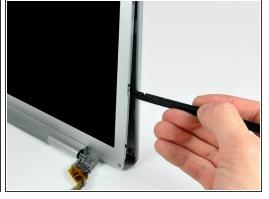
Now that the right and bottom edges of the rear bezel are slightly separated from the front bezel, use a spudger to pop the rear bezel off the tabs near the lower right corner of the display.
