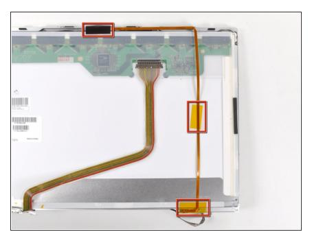
Remove the three pieces of tape securing the camera cable to the display assembly.
