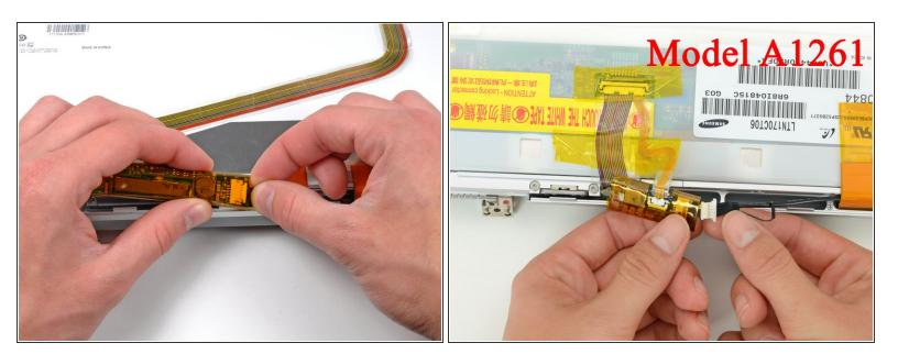
Disconnect the inverter cable by pulling its connector away from the socket on the inverter board.
