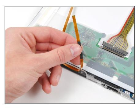
Peel the camera cable off the foam tape along the top edge of the display.
