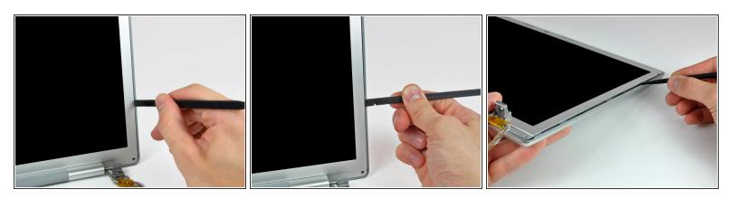
• Insert the flat end of a spudger perpendicular to the face of the display between the plastic strip attached to the rear bezel and the front bezel.
