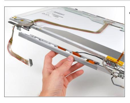
Remove the clutch assembly from the front display bezel, minding any cables that may get caught.
