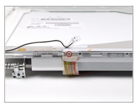
Move the display data cable out of the way to remove the Phillips screw hidden underneath.
