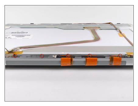
Remove the five Phillips screws securing the clutch cover to the bottom edge of the front display bezel.
