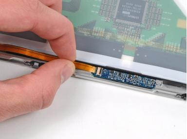
• Use the tip of a spudger or your fingernail to flip up the ZIF retaining flap on the camera cable socket at the edge of the camera board near the top center of the front display bezel.
