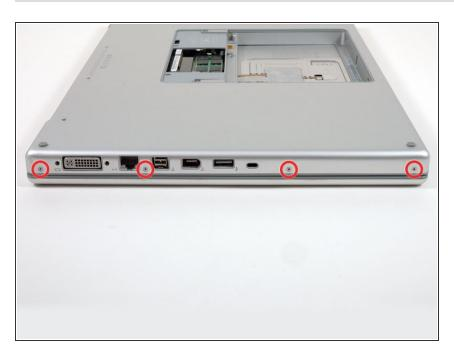
Remove the four 3.4 mm Phillips screws on the port side of the computer.
