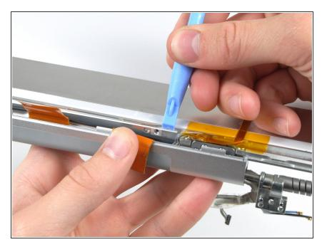
Repeat the process covered in the previous step to free the other side of the clutch assembly from the front display bezel.
