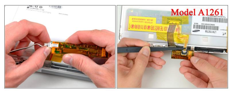
Disconnect the backlight connector from the inverter board.
