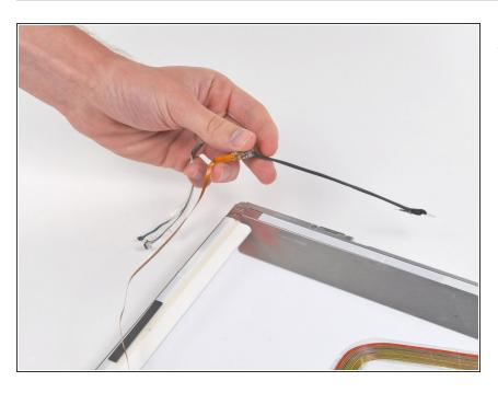
Remove the inverter/antenna cables from the display.
