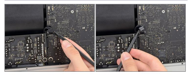
• Use the tip of a spudger to push each side of the power supply control cable connector and gently *walk* it out of its socket.
