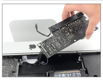
Remove the power supply from the iMac.
