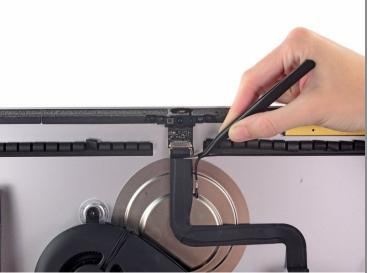
• Use a pair of <u>tweezers</u> to grasp and flip the metal retaining bracket downwards to free the iSight camera cable connector.
