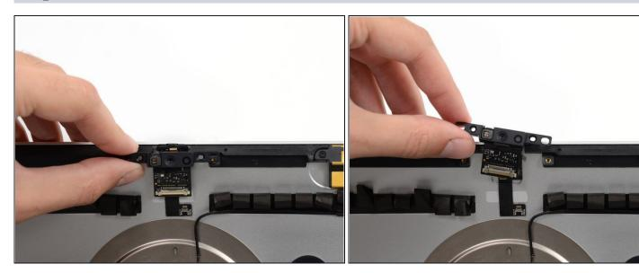
Lift and remove the camera assembly from the iMac.
