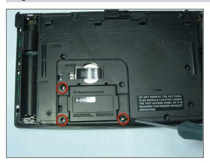
Using the same Phillips screwdriver, unscrew the remaining three 11.8mm screws.
