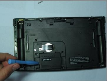
Using the Ipod Opening Tool pull up on both sides of the rectangular module while keeping the rest of the calculator flat on a surface face down
