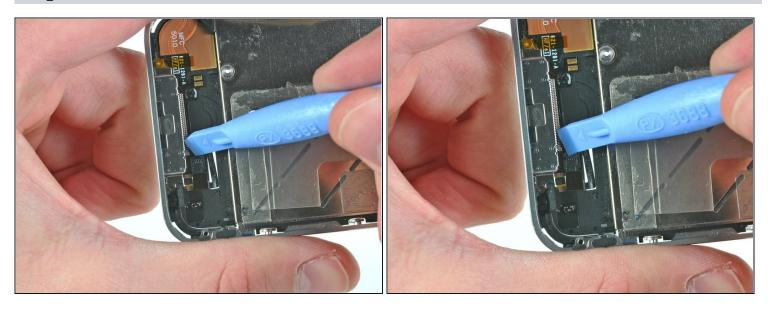
• Use the edge of a plastic opening tool to flip up the retaining flap on the home button ribbon cable.
