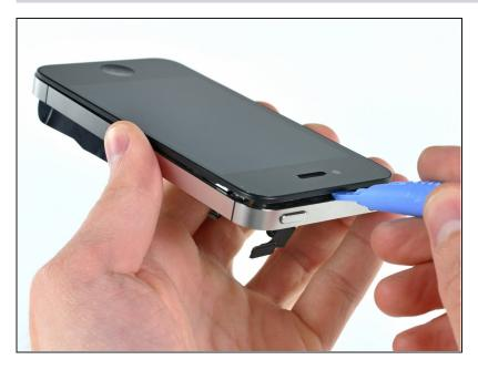
• Use the edge of a plastic opening tool to gently pry up the display assembly around its perimeter.
