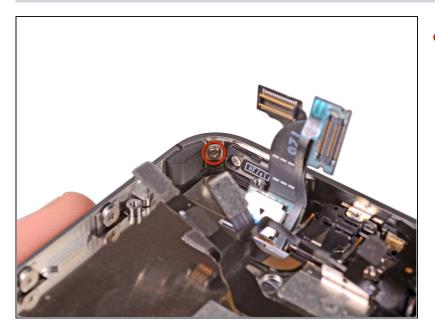
Remove the 1.5 mm Phillips screw securing the display assembly near the power button.
