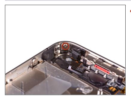
Remove the 1.5 mm Phillips screw near the lower microphone.
