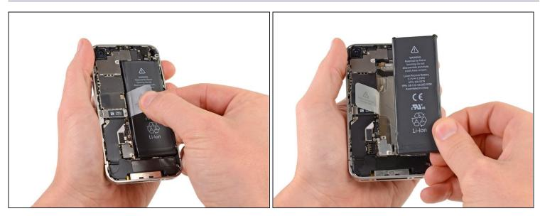
• Use the exposed clear plastic pull tab to peel the battery off the adhesive securing it to the iPhone.
