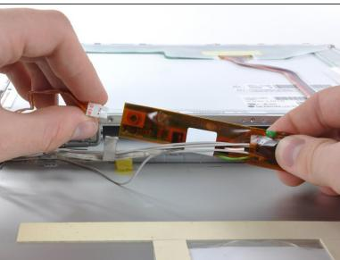
Disconnect the inverter cable by pulling the connector away from the socket on the inverter board.
