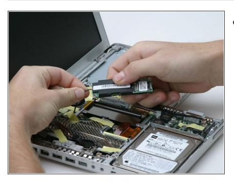
Disconnect the modem cable from the modem.
