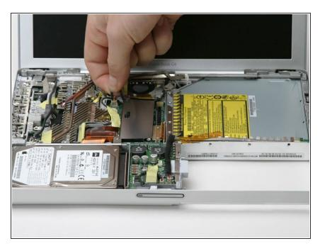
Disconnect the fan cable from the logic board.
