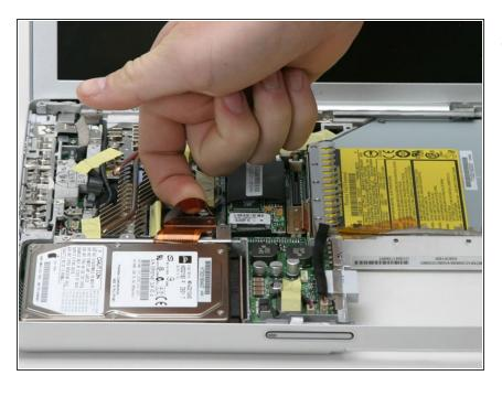
Use the orange plastic loop to disconnect the hard drive cable from the logic board.
