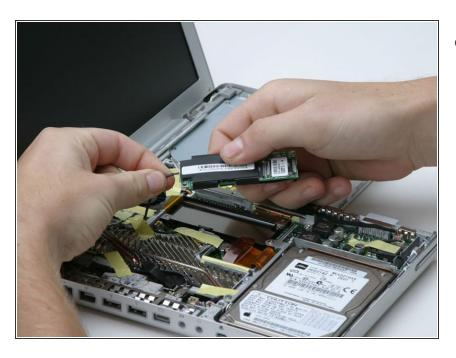
Disconnect the modem cable from the modem.
