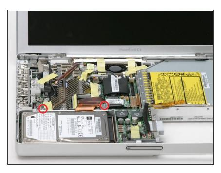
Remove the two Phillips screws from the hard drive bracket.
