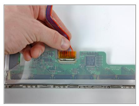
Pull the display data cable connector away from its socket to disconnect it from the LCD.
