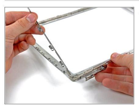
Lift the bar section of the clutch hinge a bit and remove the entire clutch hinge from the front display bezel.
