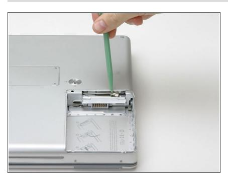
Use a spudger to disconnect the Airport antenna from the card.
