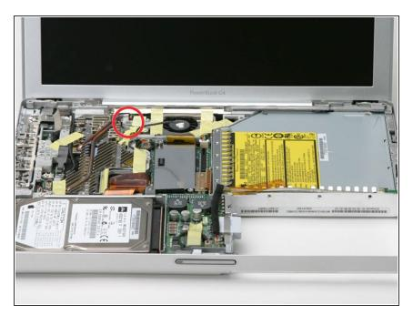
Remove the single Phillips screw fastening the inverter cable.
