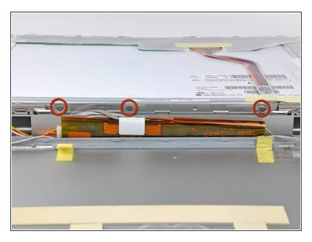
Remove the three 3.0 mm Phillips screws connecting the clutch cover to the front display bezel.
