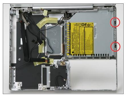
Remove the two recessed Phillips screws on the right side of the optical drive.
