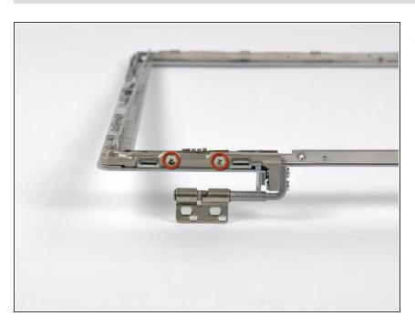
Remove the two 5.5 mm Phillips screws securing the right clutch cover to the front display bezel.
