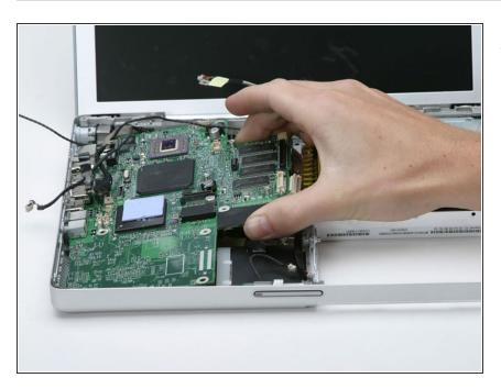
Lift the logic board partly up from the optical side.
