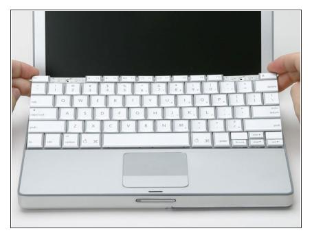
Lift the keyboard by the 'esc' and 'eject' keys and gently lift up until the keyboard is vertical.
