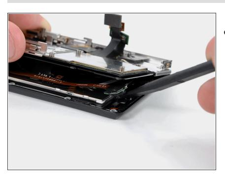
Use the flat end of a spudger to lift the board that contains the ambient light sensor and display data cable connector out of the screen housing.
