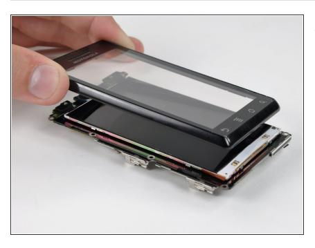
Flip the phone over and remove the front panel.
