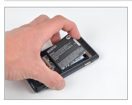
Grasp the upper left corner of the battery and lift it out of its housing.
