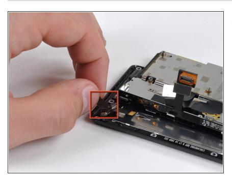
Peel off the black tape to reveal the front panel connector.
