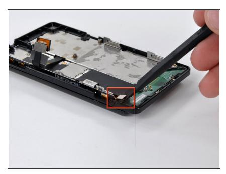
Disconnect the camera button/vibrator connector by prying it straight up off its socket on the speaker board with a spudger.
