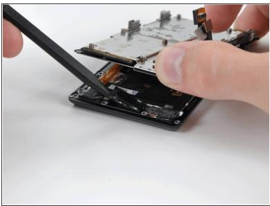
Use the tip of a spudger to lift the speaker out of the screen housing.
