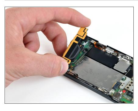
Carefully lift and remove the speaker assembly up out of the phone.
