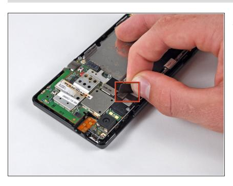
Peel the black tape covering the side button and display ribbon connectors on the motherboard.
