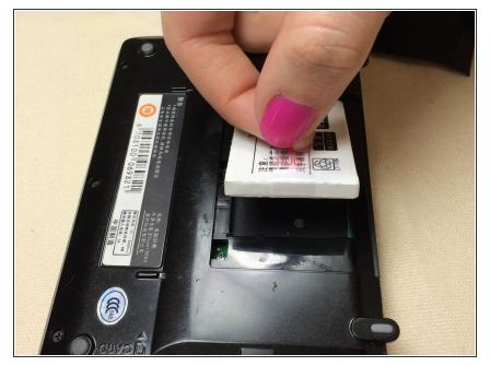
• Pull upwards on the battery tab to remove the battery from the device.
