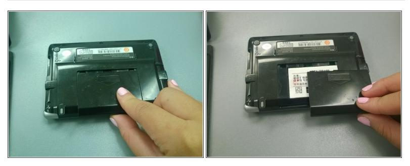
• Place your fingers on the battery cover arrow and pull the cover down and off the device.
