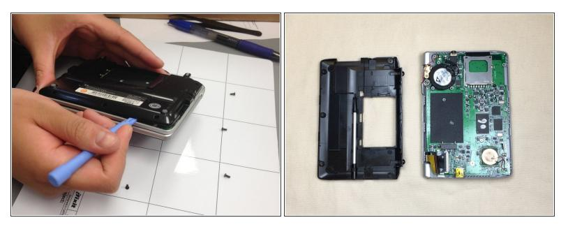
Potential for device damage: All screws must be removed before you begin this step. Do not forcefully pry apart the device with screws still in it because you may damage it.
