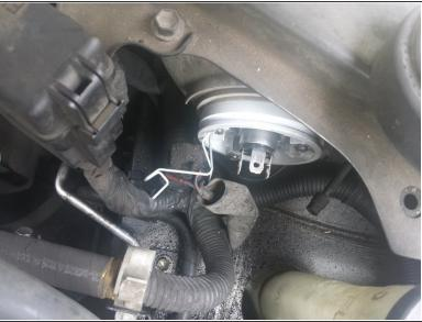
Release the bulb by pushing the metal fastener inward and then moving it upwards.
