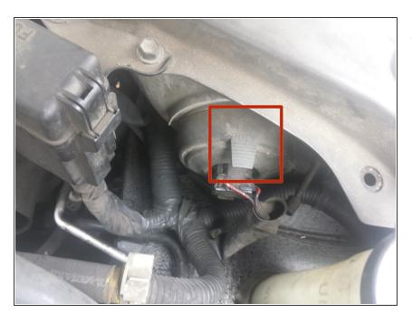
Remove the rubber cover by pulling on the tab marked "Pull Top" away from you.
