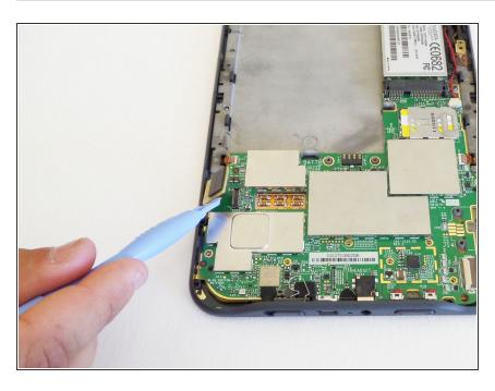
Pry the display connector straight up from its socket on the motherboard to disconnect it.
