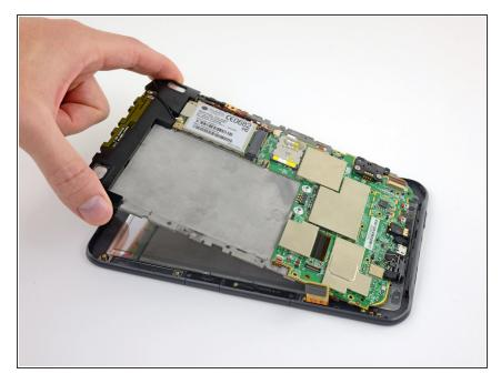
Lifting from the top edge, slide the entire motherboard and midframe assembly together away from the bottom edge of the Kindle, and remove it carefully.
