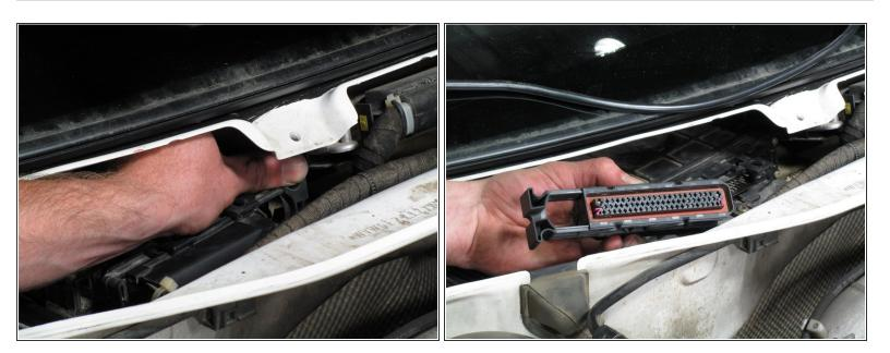
Gently unplug and lift out the automatic transmission control unit.
