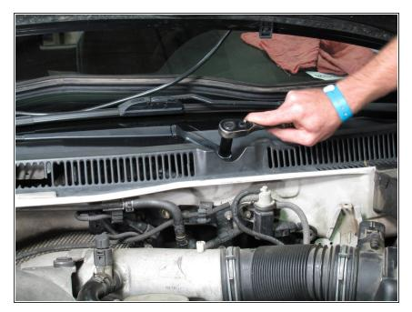
Use a socket wrench to release the passenger-side windshield wiper locking nut.
