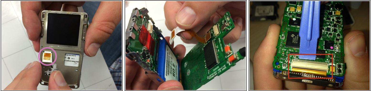
**⚠** Do not damage the ribbon tab (pictured). It is vital to the device.
