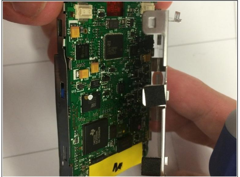
**i** No tools are needed. The prongs (pictured) will release easily to remove the back cover.
