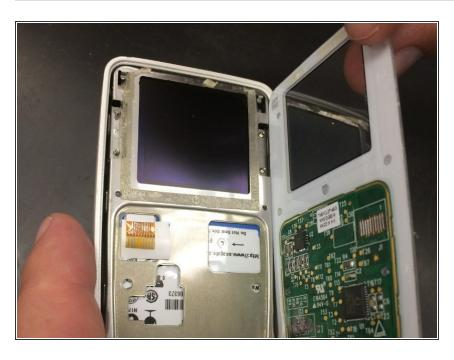
Slowly detach the front cover from the rest of the device to reveal the interior.
