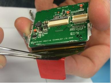
• With the tweezers, carefully pull the red strip off of the back of the screen.
