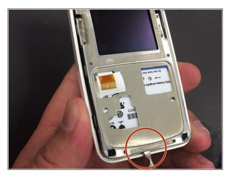
Insert the flat-head screwdriver into the notch on the bottom of the device. Pry the main board and screen from the outer shell of the device.
