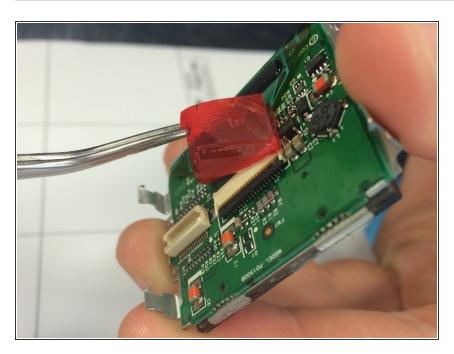
With tweezers, lightly pull down on red strip in the middle of the back of the screen.
