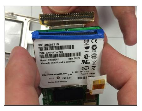
Carefully pull out the gold piece from the top of the hard drive.
