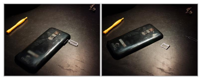
• Use a SIM eject tool to eject the SIM tray
