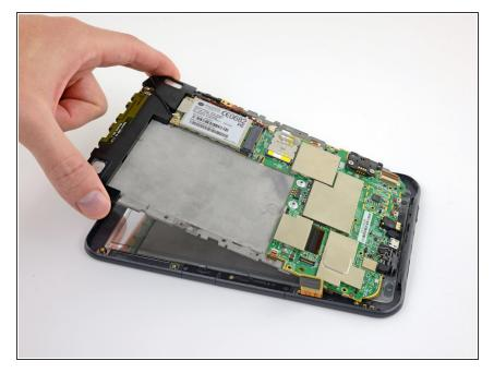
• Lifting from the top edge, slide the entire motherboard and midframe assembly together away from the bottom edge of the Kindle, and remove it carefully.
