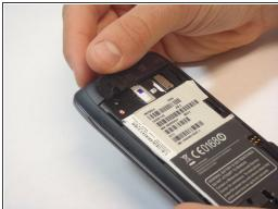
Using tweezers or your finger, lift the rubber SIM card cover to expose the card itself.
