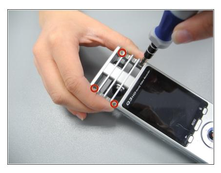
Flip the device over and remove the four screws bordering the grate of the device.
