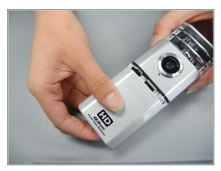
On the front of the device, slide the battery compartment cover off by pushing inward and sliding downward.
