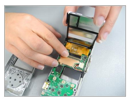
Gently flip the black clip up attaching the ribbon of the screen to the circuit board.
