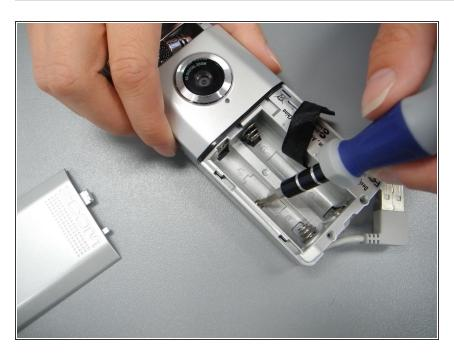
Remove the final screw from the bed of the battery compartment.
