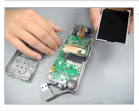
Gently slide the ribbon from the circuit board, removing the screen.
