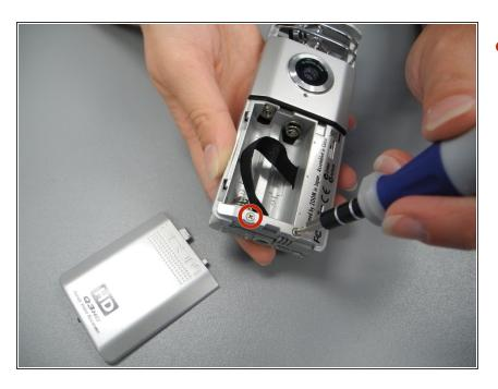
Remove the two screws from the lip of the battery compartment.
