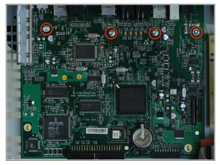
Unscrew the four screws on the motherboard with a T10 screwdriver.
