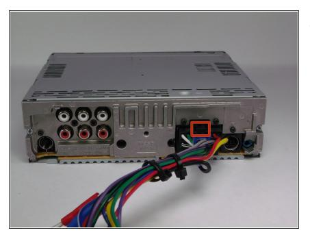
• Locate the clip on the wiring harness.
