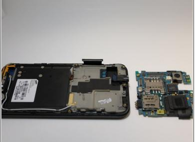
• Lift the motherboard out of the base of the phone.
