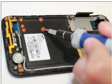
Remove the eight screws using the #00 screw driver.
