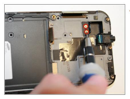
Remove screws using the #00 screwdriver.
