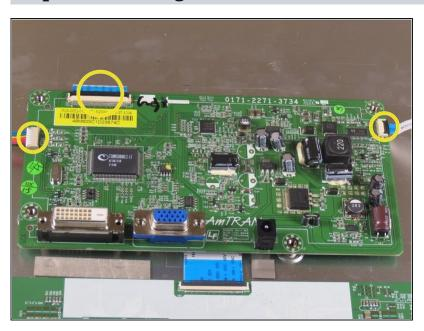
The following steps circled in yellow are the locations for detaching the three connectors shown in the picture.
