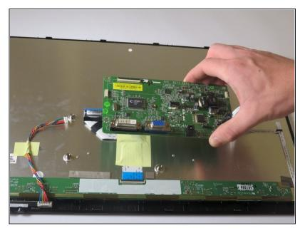
• Gently lift the motherboard to remove it from the monitor.
