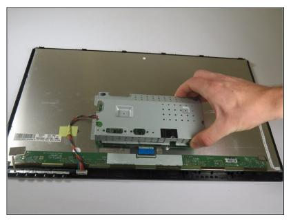
• Gently lift the motherboard casing from the monitor.
