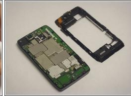
Separate the housing from the motherboard.
