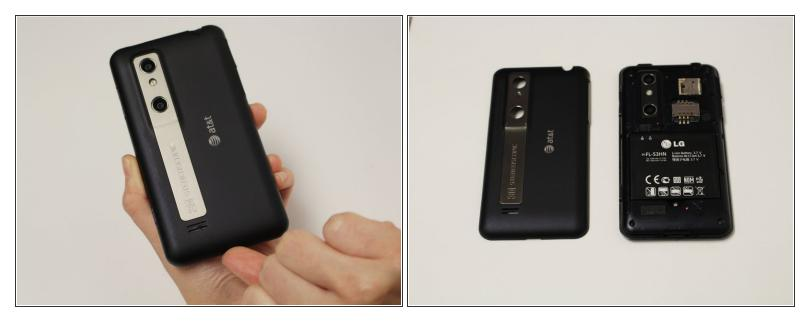
• Pry the back cover off of the phone with your fingernail. There is a notch located at the bottom of the phone for improved leverage.
