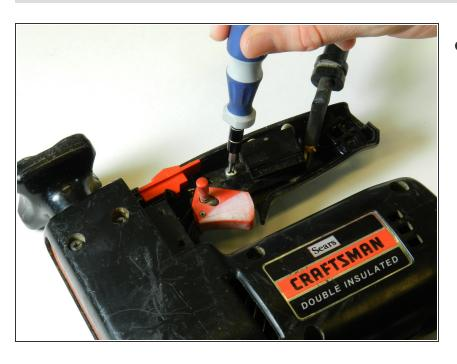
Remove the 1/2" Phillips screw that is securing the switch using a Phillips #1 screwdriver.
