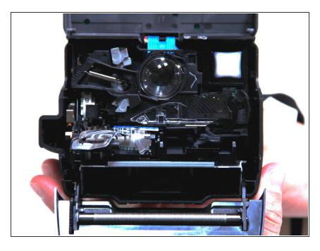
Once the front assembly is removed, the primary lens should be exposed without any trouble.
