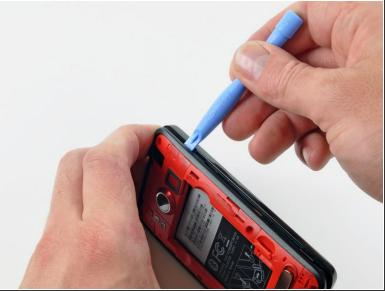
• Insert the iPod opening tool between the rear inner frame and its plastic surround and pry up at several points along the left edge of the Evo.
