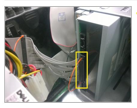
Gently remove the CD/DVD and power cables from the back of the optical drive
