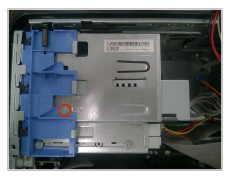
Using a Phillips #1 screwdriver, remove the screw connecting the optical drive to the drive bay.
