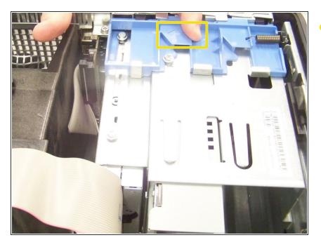
Slide the blue latch downward until the panel can be removed from it's hinges.
