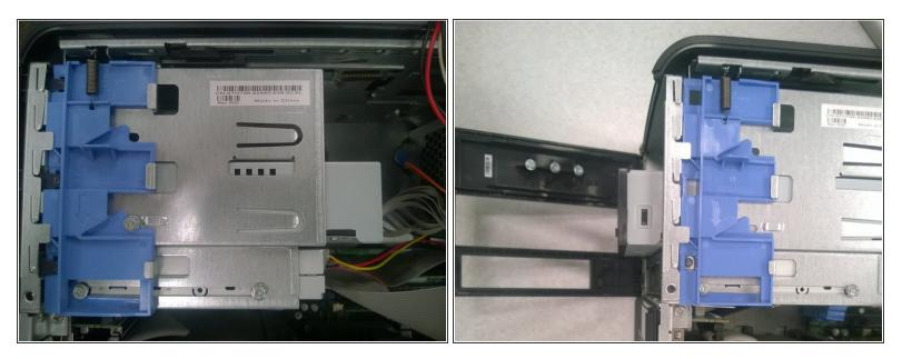
• To remove the optical drive from the drive bay, slide the drive towards the front of the computer.
