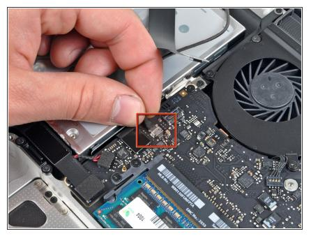
Disconnect the camera cable by pulling its connector away from the socket (toward the optical drive) on the logic board.
