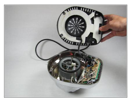
Lift the back panel up, sliding it along the power cord.
