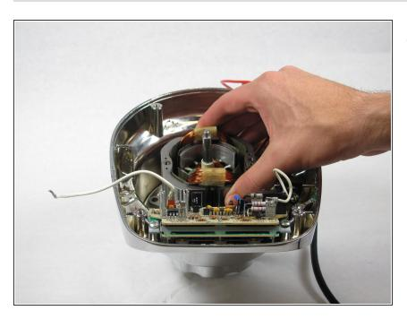
Lift the motor up out of the chassis.
