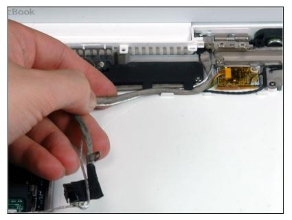
• Deroute the silver microphone cable and gray display data cable from the tabs at the bottom of the subwoofer.
