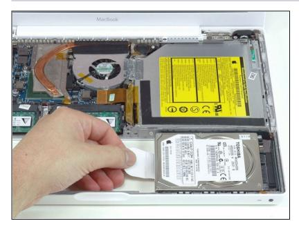
• Grasp the white plastic tab attached to the hard drive and pull it to the left, removing the hard drive from the computer.
