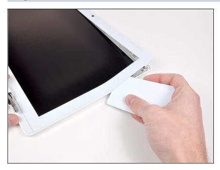
• Next, free the five tabs securing the display bezel on the right side.
