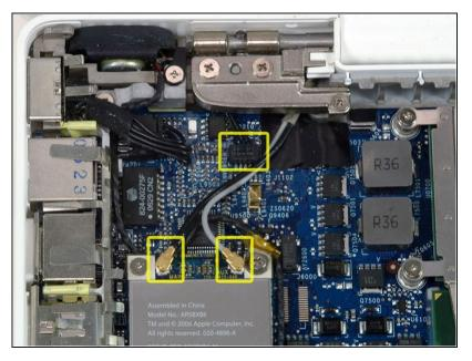
• Disconnect the two antenna cables from the Airport card, and the black inverter cable from the logic board. (Pull vertically on all three.)
