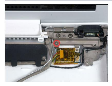
Remove the single 3.2 mm Phillips screw securing the ground loop in the display data cable located just above the Bluetooth board.
