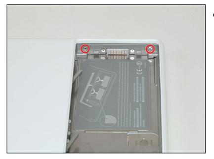
Remove the two 6 mm Phillips #00 screws from either side of the right wall of the battery compartment (not the ones closest to the battery connector).
