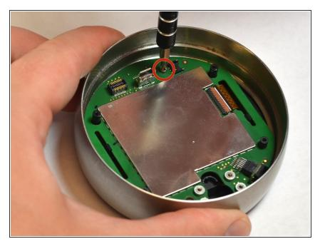
Remove the 4 mm screw from the motherboard using a #0 Phillips screwdriver.
