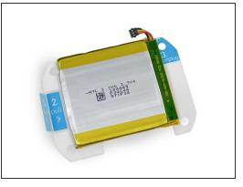
Grasp the battery with your fingers and pull directly away from motherboard to separate the battery from the display.
