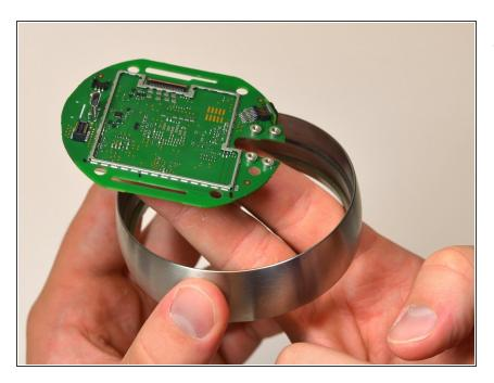
Using one hand to hold the steel ring, carefully lift the motherboard out of the ring using the other hand.
