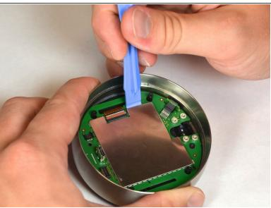
Remove the EMI shield from the motherboard using a plastic opening tool.
