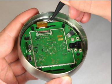
Unsnap the LCD ribbon from the motherboard gently using tweezers.
