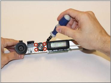
• Once the area where the camera is found is uncovered, use the T5 Torx Screwdriver to remove the four 1.9x10.2 mm screws.
