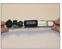
• First step is to make sure that the inner compartment containg the camera is separated from the outer casing.
