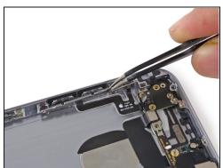
• Pull the hold switch and volume control button brackets away from the rear case to allow access to the button covers.
