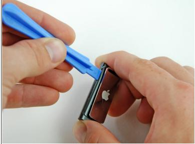
Insert an iPod opening tool into the newly widened gap, and pry the rear case up and away from the front case.
