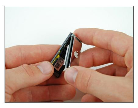
Lift the bottom of the rear case and remove it from the rest of the iPod.
