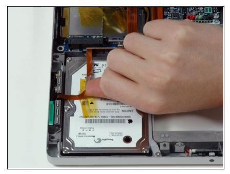
Peel up the orange ribbon cable taped to the top of the hard drive.
