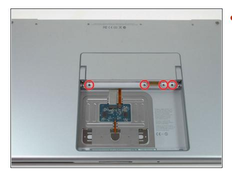
Remove the four identical Phillips 3.4 mm screws from the memory door. These screws have 4 mm diameter heads rather than the 3 mm heads on the body screws.
