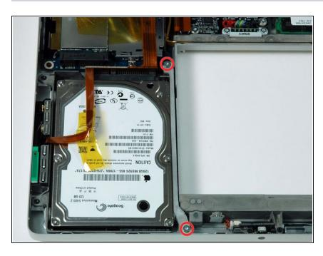
Remove the two T6 Torx screws securing the hard drive retaining bracket to the lower case.
