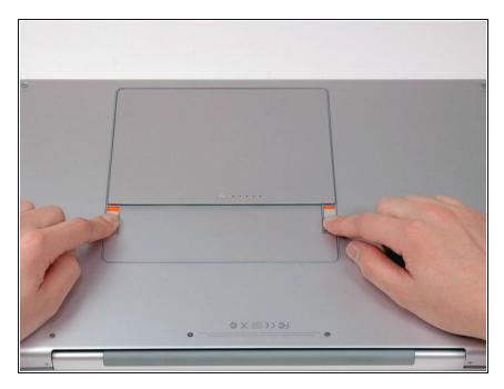
Use your fingers to push both battery release tabs away from the battery and lift the battery out of the computer.
