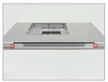
Rotate the computer 90 degrees and remove the two Phillips screws from the rear of the computer.
