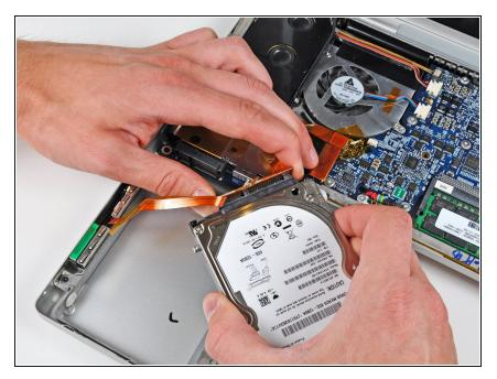
Disconnect the hard drive cable by pulling its connector away from the hard drive.
