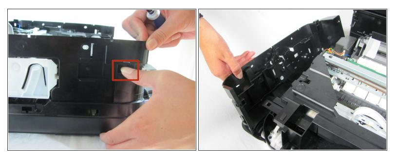
Press down on the clip on the left side of the printer until it clicks, and pull the panel free.
