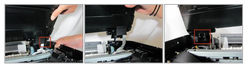
Remove the scanner by pulling the side panels out until the scanner pin is free. Set the scanner aside.
