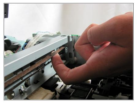
• Remove the cord by pulling upwards on it and unhooking it from the pulleys on either end.
