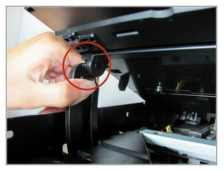
Unhook the lid support by sliding the hook down and to the left. Make sure the support is fully disconnected before proceeding.
