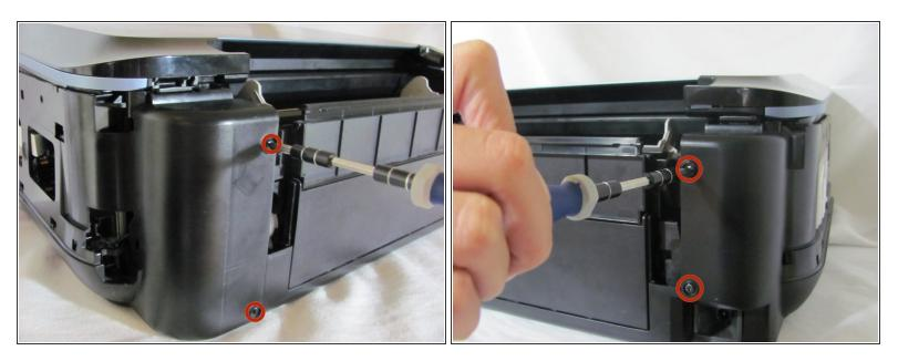
• Remove the four black screws on the back panels from both the left and right side.
