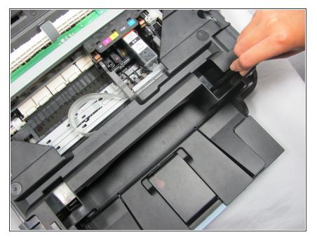
Remove the plastic cover by depressing the clip located on the right side of the printer. Press the clip inwards until it clicks, and then lift the cover upwards and off the printer.
