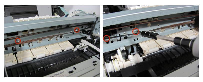
Unscrew the three screws holding the rail.
