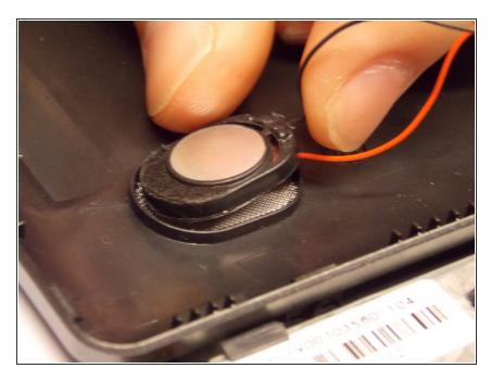
Apply a small amount of adhesive to the new speaker, and place it into the housing on the back panel.
