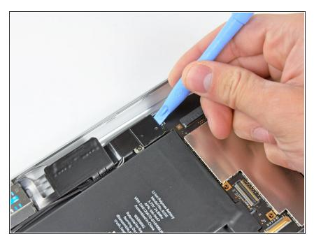
• Use the edge of an iPod opening tool to pry the SIM board connector up off it socket on the logic board.
