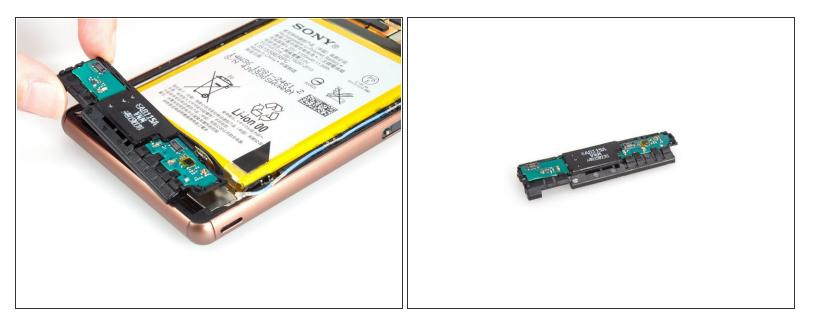
• Remove the loudspeaker assembly finally. Be careful with the flex beside assembly.
