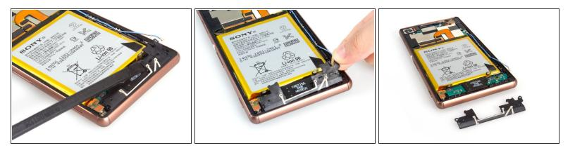
• Remove the securing cover. It's thin and weak, please be careful when remove it.
