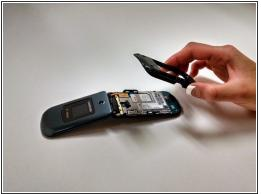
Using the plastic opening tool, work around the edge of the black plastic cover until it pops off
