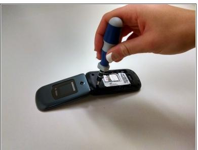
Remove the four Phillips 1.0mm #0 screws
