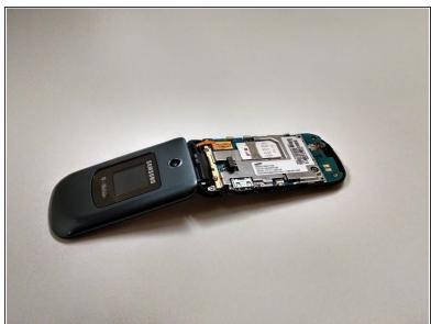
Remove side buttons by lifting them off the board
