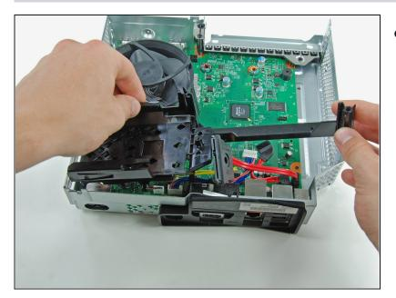
• Lift the hard drive bracket out of the metal frame.
