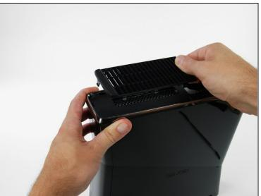
Remove the bottom vent by lifting it away from the bottom bezel.
