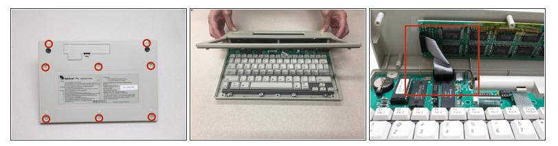
Removing the lithium coin battery will erase existing files. Make sure all important files have been safely transferred to another device before attempting to remove the lithium coin battery.
