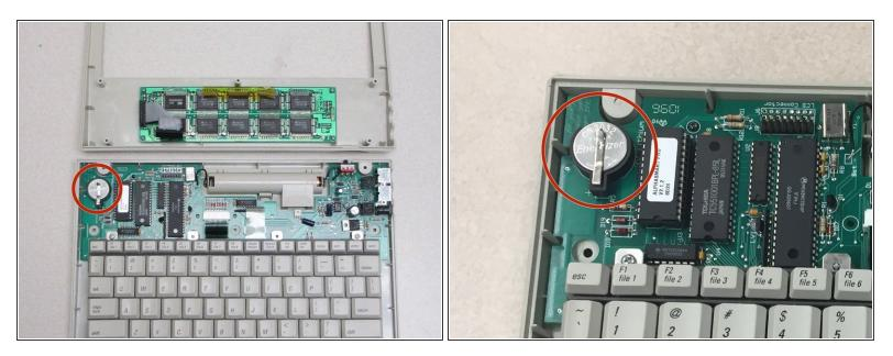
• With the front panel removed, locate the lithium coin battery at the top left corner of the motherboard.
