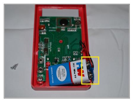
After removing the outer casing and motherboard of the device, locate the attachment site of the battery to the motherboard.
