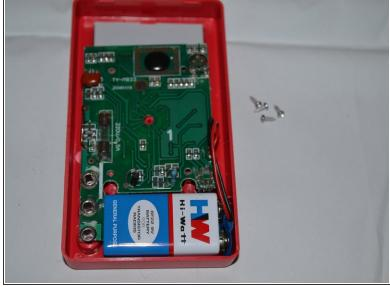
• Remove the four 7mm Phillips screws holding the circuit board in place.
