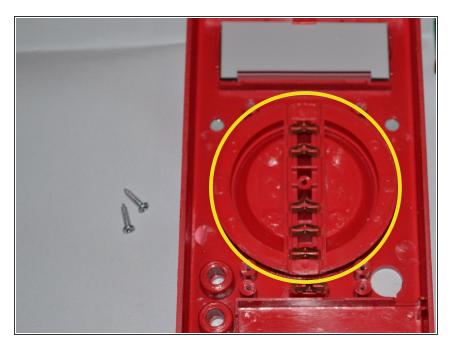
The dial is located in the central part of the device.
