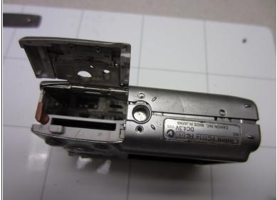
Slide the battery out of the battery compartment.
