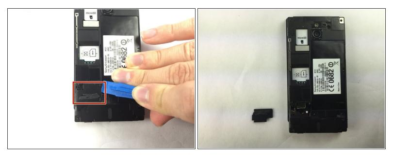
Locate the black cover on the bottom left of phone. Use an opening tool to pry up and remove the black cover.
