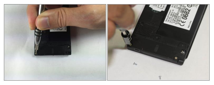
Locate and remove the 2 additional screws, using the 26 Bit Kit, that are revealed. These are marked as shown.
