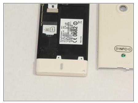
Push on cover away from you. You should hear a snap or pop. This will let you view the battery and sim/sd card slots. Then lift the cover off.
