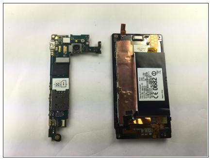
• Use the spudger and slide it under the top left of the board then lift the board straight up. The board should come up very easily.
