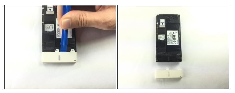
• Pry off the bottom white cover by using the opening tool as a lever.
