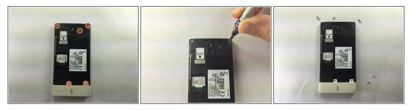
• Locate and remove the five (5) screws on the phone, using the 26 Bit Kit. The screws are at the top and the bottom of the phone as shown.
