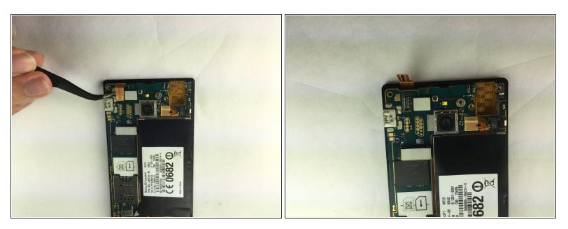
• Use the tweezers to lift up on the circuit located at the top left.
